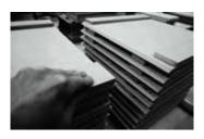
Planters & Furniture Image'ln are manufactured in fibre cement Eterboard® HDNT (High density new technology) in thickness of 10 or 15 mm depending on the product sizing. This material, standed out through high stability, is crafted in cutting and gluing. Then It is laquered and varnished for an optimal coat.
