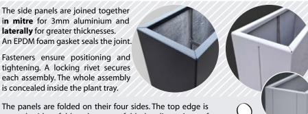
treated with a fold and counter-fold, the dimensions of which are adjusted according to the planter's size. The bottom fold forms a hollow joint with the floor. Its slightly open angle directs water run-off towards the underside of the pot.
